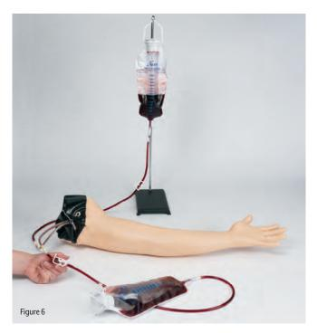
6. Once the system is filled, close the clamp on (resting) fluid supply bag and leave (hanging) fluid supply bag clamp open. The arm is now fully pressurized and can be used palm up or down. (*See figure 6.*)
