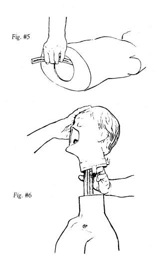
3. Stand torso upright and remove mouth/nose piece from face. Remove HEAD by unsnapping the two tab strips and lift from torso with valve and tubes attached. (Fig. #6)
